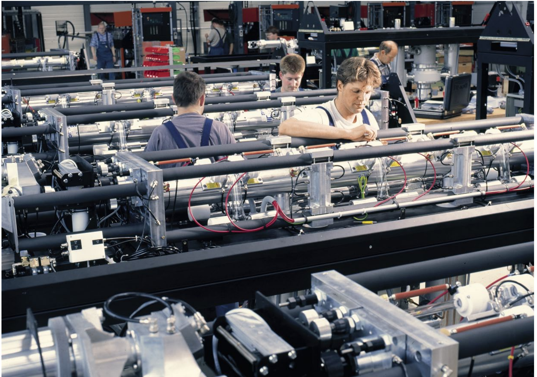
▲ Resonator assembly until 1999 Bystronic produced only valve excitation lasers
