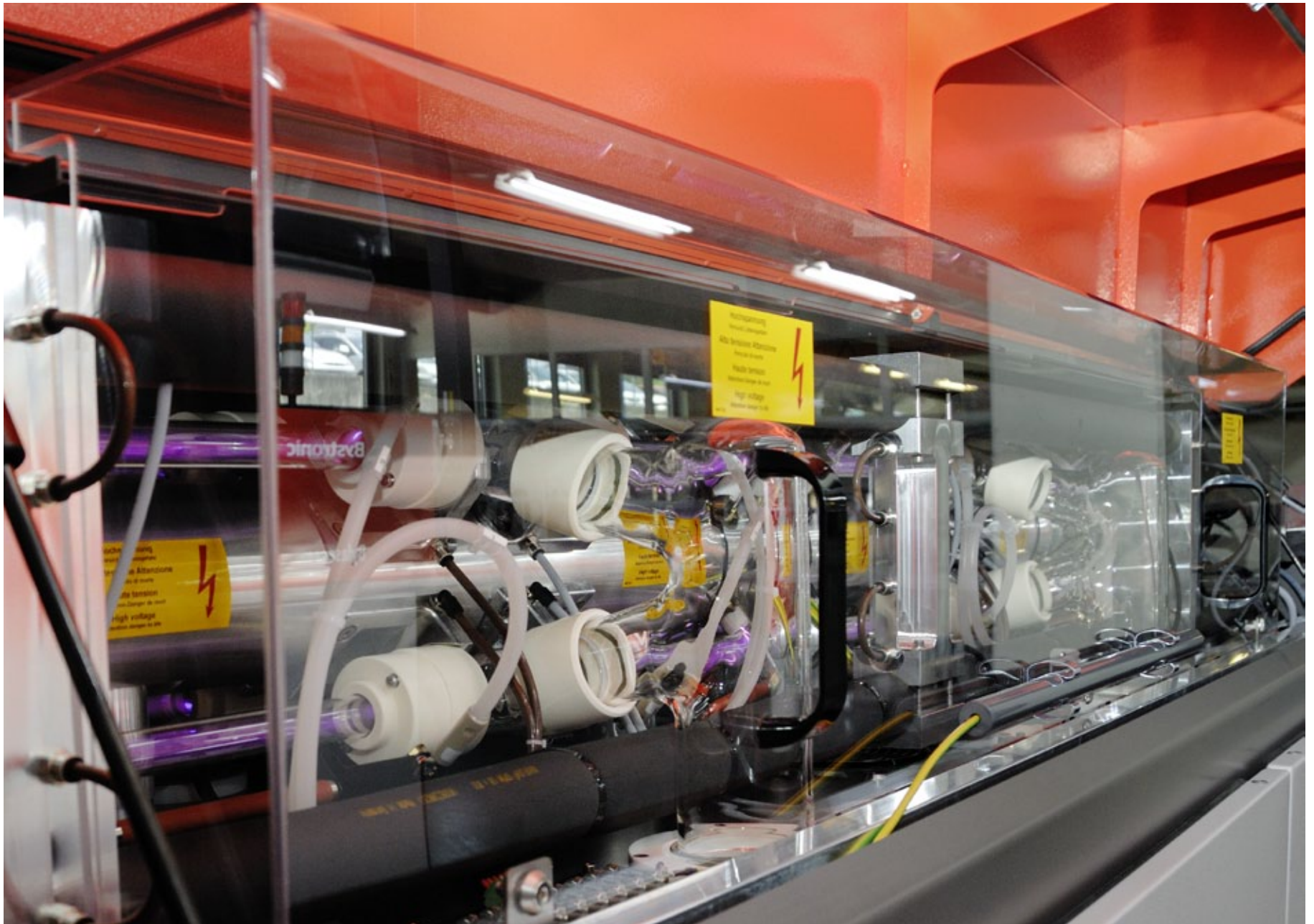
▲ The second-generation laser source was based on semiconductor excitation
