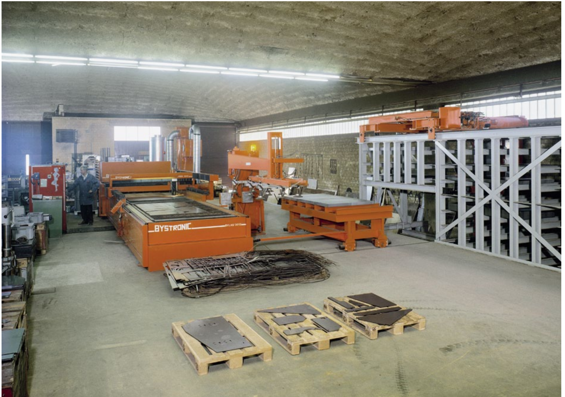
▲ Bystronic bought a 500 watt laser in England, assembled it on one of their glass cutting machines and started to cut sheet metal at Samro.
